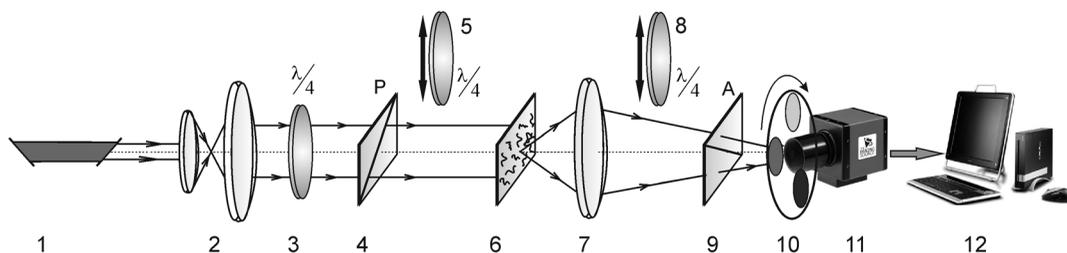
**Fig. 2** Optical scheme of laser polarization autofluorescent Stokes polarimeter.
