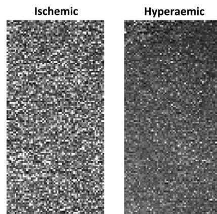
**Fig. 5** Raw speckle images from the surface of a finger tip. The left panel is taken when blood flow to the finger tip is temporally stopped. The speckle pattern shows high contrast between white and dark speckles. The right panel was taken immediately after blood flow was restored to the finger. The speckle pattern is blurred due to the motion of the red blood cells in the flowing blood.
