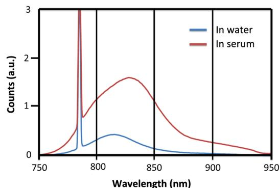
**Fig. 2** Fluorescence emission spectrum of ICG excited at 785 nm in both aqueous solution and serum at a weight volume of 0.075 mg/ml. A signal enhancement is observed in serum due to protein binding and improved fluorescence quantum yield. A broader and more red-shifted emission is observed in serum compared to water.
