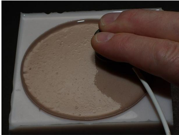
**Fig. 1** Measurement on a two-layered PDMS phantom. The thin epidermis-mimicking coffee phantom is placed on top of the thick dermis phantom, and the measurement probe is held in place by the fingers. Small air-bubbles and/or surface inhomogeneities can be observed in the two-layered phantom.
