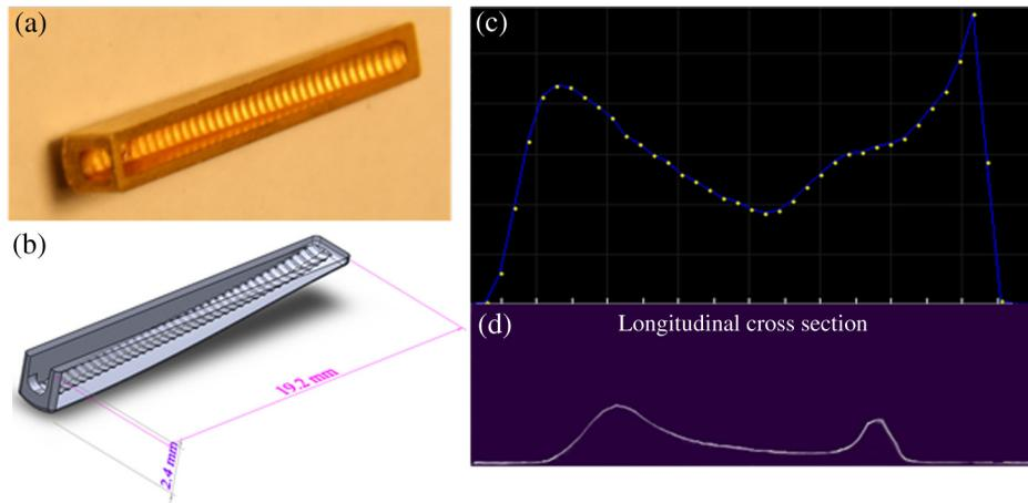
**Fig. 3** (a, b) Photograph and diagram of reflective insert with “staircase” geometry placed in lower jaw of laparoscopic prototype; (c) simulation of spatial beam profile; (d) experimental results for spatial beam output of probe.
