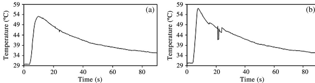
**Fig. 10** Temperature versus time graphs for outside surface of (a) lower and (b) upper jaws. The exact locations can be seen labeled as cursor 1 and 2 in Fig. 9. The abrupt drop in temperature shown in (b) at  $t = 25$  s is due to movement of the jaw to remove the vessel after laser irradiation.
