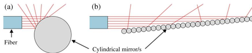
**Fig. 1** (a) Side view diagram of fiber illuminating top half of single cylindrical mirror. (b) Washboard-style, multiple cylindrical mirrors arranged in a staircase, creating a longer linear beam directed at 90 deg. Additionally, the shorter height of the optics meets design constraints of the laparoscopic probe jaw.
