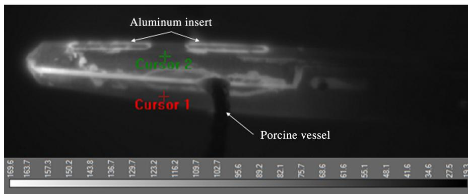
**Fig. 9** Thermal image of jaw acquired at time of peak detected temperature inside the jaw ( $>135^{\circ}\text{C}$ ). The figure uses a false color image scale, with lightest color corresponding to highest temperature ( $>135^{\circ}\text{C}$ ) and darkest corresponding to lowest temperature ( $20^{\circ}\text{C}$ ).
