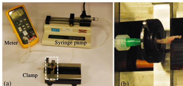
**Fig. 5** (a) Burst pressure experimental setup; (b) an iris was used to clamp vessels to a needle, which were then filled with deionized water until the seal burst. Pressure before burst was recorded using a pressure meter.
