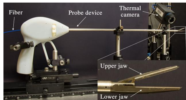
**Fig. 4** Prototype device using traditional 5-mm OD Maryland jaw configuration. Insert shows magnified view of upper and lower jaws on the laparoscopic device. Thermal camera was used for noninvasive temperature mapping during the procedure.
