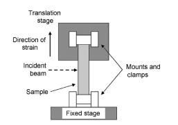
Fig. 5 Image from Ref. 114. Apparatus to create birefringent phantoms.
