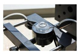
**Fig. 6** Optical phantom from Ref. 124. The custom-built ocular model. Glucose concentration in the anterior section is varied through the two infusion tubes.
