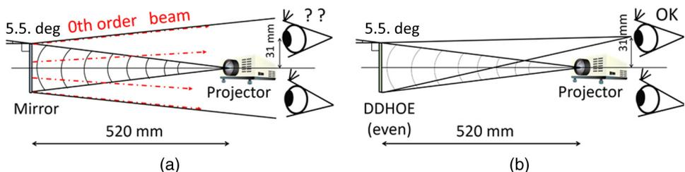
**Fig. 7** Top view of glasses-free binocular display: (a) with mirror and (b) with DDHOE.
