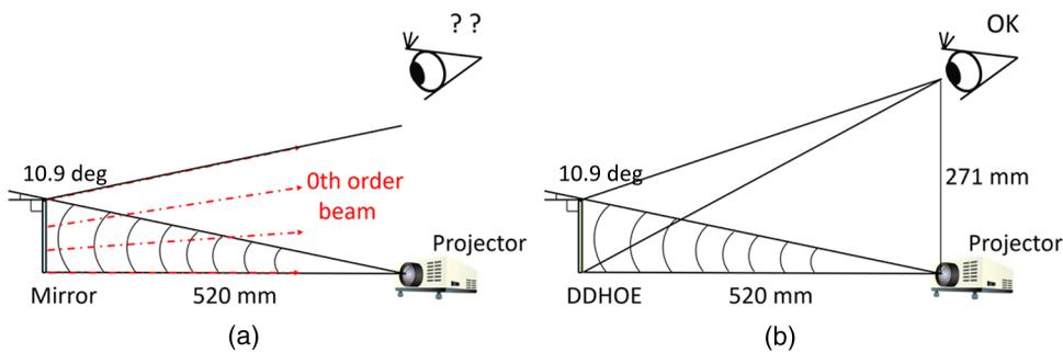
**Fig. 6** Side view of glasses-free binocular display: (a) with mirror and (b) with DDHOE.
