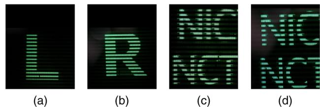
**Fig. 9** Optical reconstruction of binocular display: (a) from left, (b) from right, (c) from left, and (d) from right.
