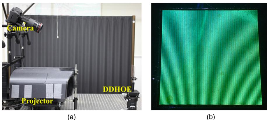
**Fig. 11** Light field display using DDHOE screen: (a) experimental setup and (b) prototype light field screen.
