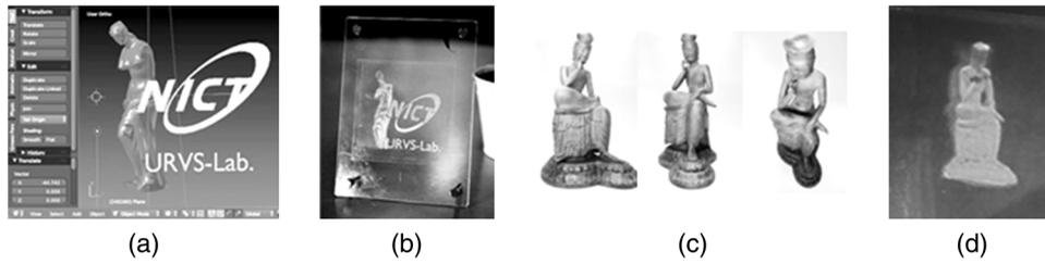
**Fig. 4** Virtual scene and real object converted into hologram and printed by hologram printer: (a) virtual objects, (b) printed hologram of virtual objects, (c) real object, and (d) printed hologram of real object.
