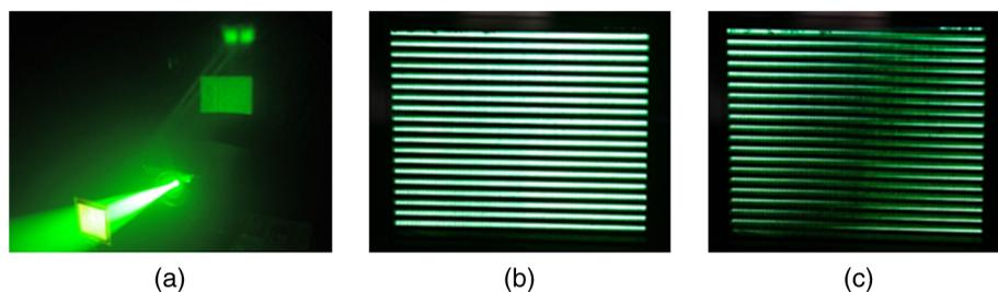
**Fig. 8** Reflection function of the printed DDHOE: (a) light converges at eyes, (b) from left eye, and (c) from right eye.
