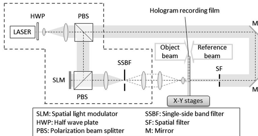
Fig. 1 Schematic of hologram printer.
