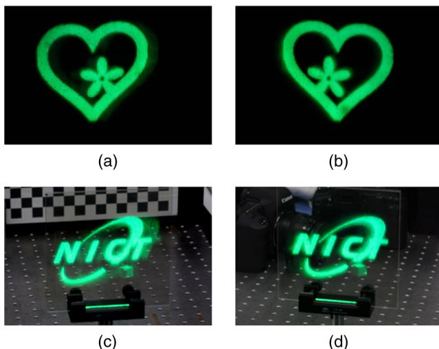
**Fig. 12** Reconstructed 3-D images using the DDHOE light field screen.
