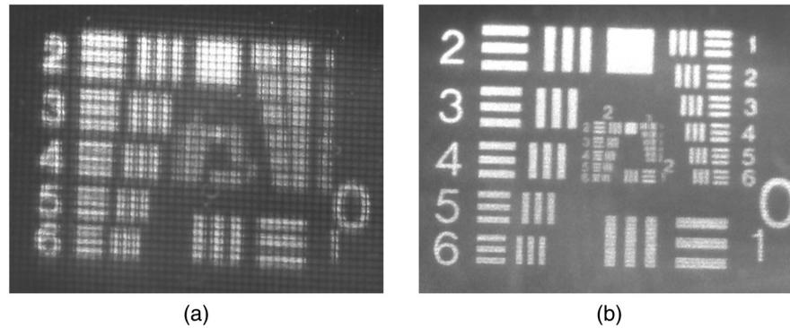
**Fig. 3** Magnified overlapped and nonoverlapped images printed using the wavefront printer: (a) 648- $\mu\text{m}$  nonoverlap image and (b) 648- $\mu\text{m}$  image printed with 324- $\mu\text{m}$  overlap.
