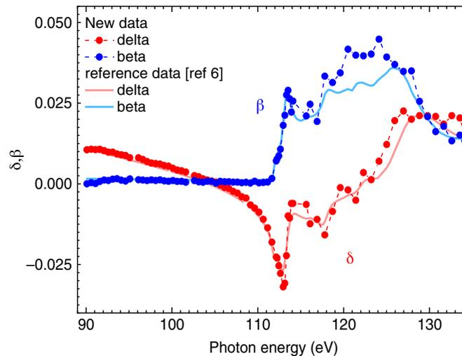
**Fig. 6** Derived optical constants of beryllium in the energy range 90 to 134 eV from [Mo/Be]  $\times$  25 ML structure (sample\_02) by combining at-wavelength reflectometry in x-ray and EUV energy range (circles). Solid lines are reference data from Ref. 7.
