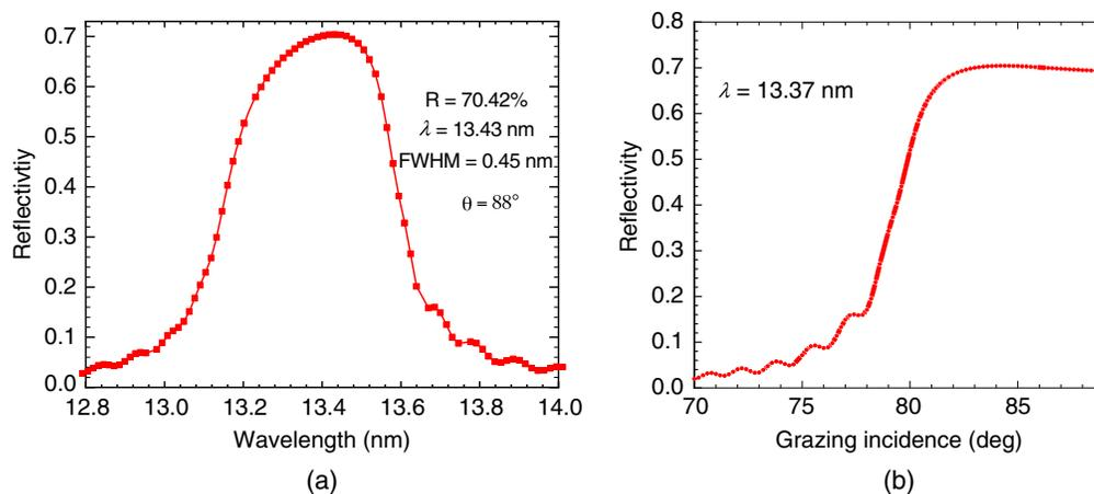
**Fig. 3** Measured reflectivity of the  $[\text{Mo/Be/Si}] \times 110$  multilayer (sample\_01) at EUV wavelengths. (a) Spectral dependence in near-normal incidence and (b) angular dependence at 13.37 nm.
