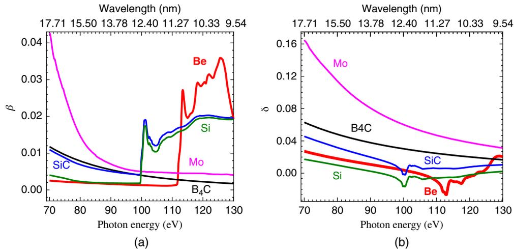
**Fig. 1** Optical constants of bulk beryllium in comparison to the commonly used low-Z materials B<sub>4</sub>C, SiC, and Si. (a) Absorption constants and (b) refractive optical constants.<sup>6</sup>
