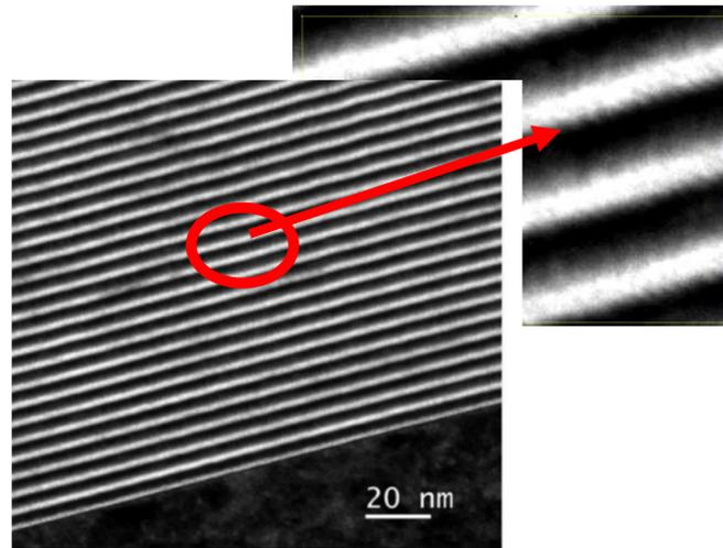
**Fig. 2** High-resolution bright field transmission electron microscopy image of Mo/Be sample to demonstrate formation of interlayers at interfaces. The ML sample was deposited in the same sputtering machine under similar deposition conditions to the samples discussed in this work.
