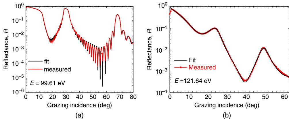
**Fig. 5** EUV measurements and corresponding fits of sample\_02 (a) at 99.61 eV and fit, (b) at the 121.64 eV. The layer and interlayer thicknesses are taken from the results of the XRR data in Fig. 4.
