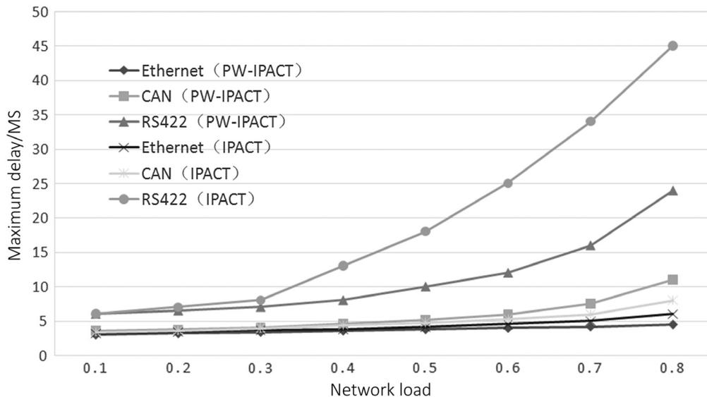
Fig. 3 Maximum data delay of the IPACT algorithm and PW-IPACT algorithm.
