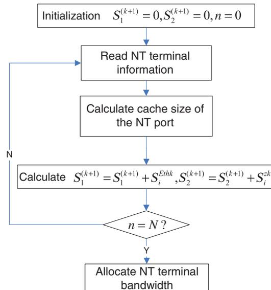
Fig. 2 NC controller bandwidth allocation algorithm flowchart.
