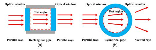
Fig. 3 Schematic diagram of the parallel rays through (a) rectangular pipe and (b) cylindrical pipe in the Schlieren apparatus.
