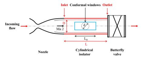
Fig. 11 Schematic configuration of wind tunnel test with the cylindrical isolator.
