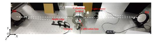
Fig. 18 Z-type Schlieren measurement system.
