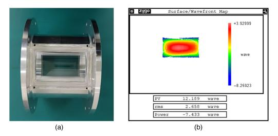
Fig. 17 (a) Cylindrical isolator with conformal optical windows and (b) interferometric measurement result.<sup>20</sup>
