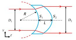
Fig. 4 Optical design model of the conformal window.
