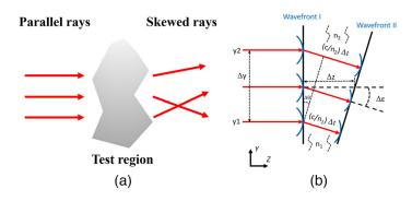
**Fig. 1** Description of light deflection phenomenon through inhomogeneous medium: (a) the deflection of the parallel rays passing through the test region and (b) the simplified physical model of the refractive light beam based on refractive index gradient on the y direction.
