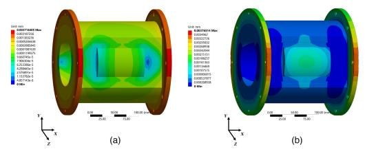
**Fig. 13** Deformation results of the isolator pipe with the (a) silica conformal optical windows and (b) acrylic conformal optical windows.
