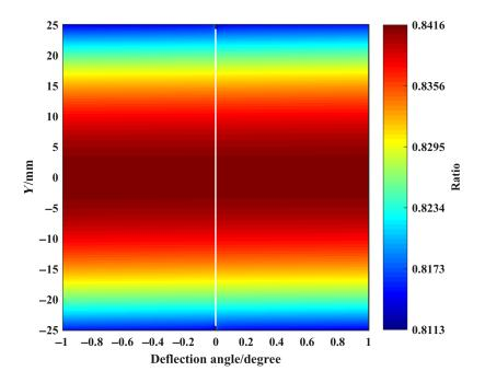
**Fig. 8** Ratio of the emergent angle  $\theta'$  to the deflection angle  $\theta$  along the Y direction.
