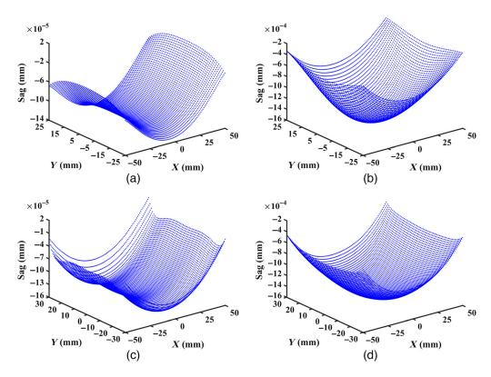
**Fig. 14** Deformation sag of the (a) inner and (c) outer surfaces of the silica conformal windows and the (b) inner and (d) outer surfaces of the acrylic conformal windows on the +Z side.
