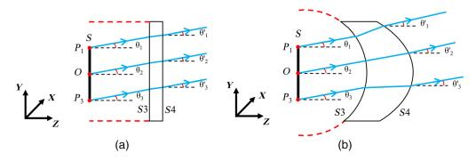
Fig. 7 Two-dimensional model of light deflection through (a) the plane window and (b) the conformal window.
