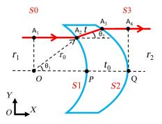
Fig. 15 Two-dimensional structure diagram of the conformal optical window.
