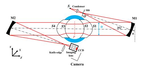
Fig. 5 Z-type Schlieren imaging system with conformal optical windows.
