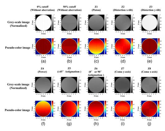
Fig. 6 (a)-(j) Imaging effects of different kinds of aberrations in the Schlieren imaging system.
