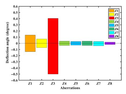
Fig. 10 Comparison diagram of maximum value of minimum acceptable absolute deflection angle of different aberrations.
