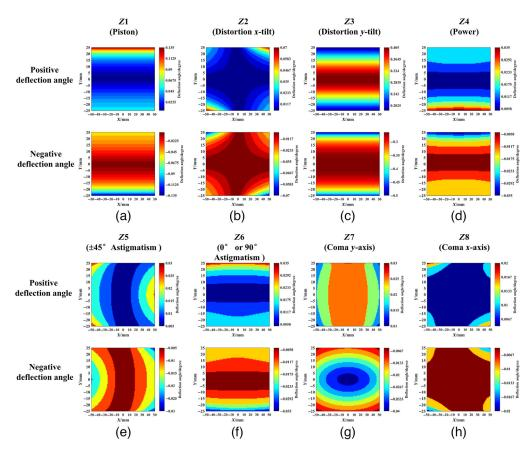
Fig. 9 (a)–(h) Acceptable minimum absolute deflection angle with a positive and negative deflection angle in the whole observation area with different window aberrations.
