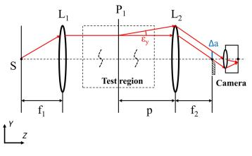
Fig. 2 Deflection of the parallel light in the Schlieren apparatus.
