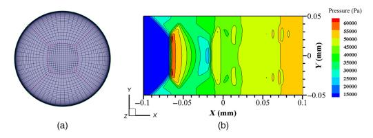
Fig. 12 (a) Grid distribution of the isolator and (b) the distribution of the static pressure of the cross section in the middle of the isolator.
