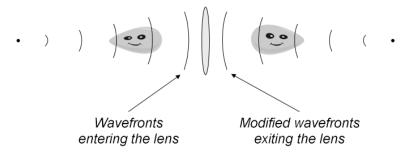
Physical optics shows us how a lens modifies the wavefronts of light to create an image.
