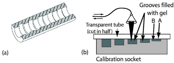
**Fig. 1** (a) Sketch of calibration socket.<sup>5</sup> (b) Simplified drawing showing cross section of calibration socket with transparent tube in place. A and B represent the interfaces responsible for the interference displayed in the spectrum. Groove depths are greatly exaggerated in both (a) and (b).
