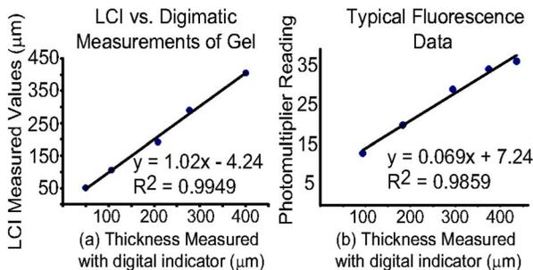
**Fig. 4** Comparison of gel thickness measurement linearity for (a) LCI-based system and (b) clinical fluorescence-based system. Note that the LCI system achieves excellent response without the need for an exogenous contrast agent.
