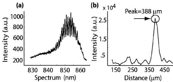
**Fig. 3** (a) Spectral data from the 388- $\mu\text{m}$  groove. (b) Correlation function obtained by FT of spectral data. The sharp peak at 388  $\mu\text{m}$  corresponds to a 277- $\mu\text{m}$  optical thickness of the gel sample.
