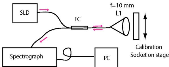
**Fig. 2** Common path LCI system. FC: Fiber coupler, L1: Lens.
