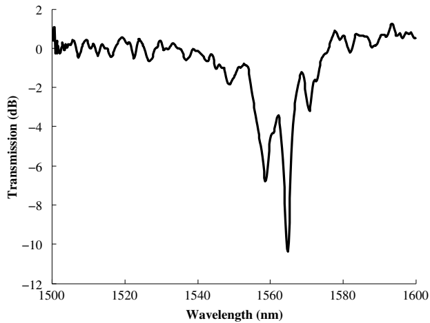
Fig. 7 Normalized spectrum of MZ configuration in the D-shaped fiber (1-nm resolution).
