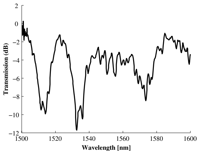
Fig. 8 Normalized spectrum of two LPGs at 1510 and 1530 nm in the D-shaped fiber (1-nm resolution).
