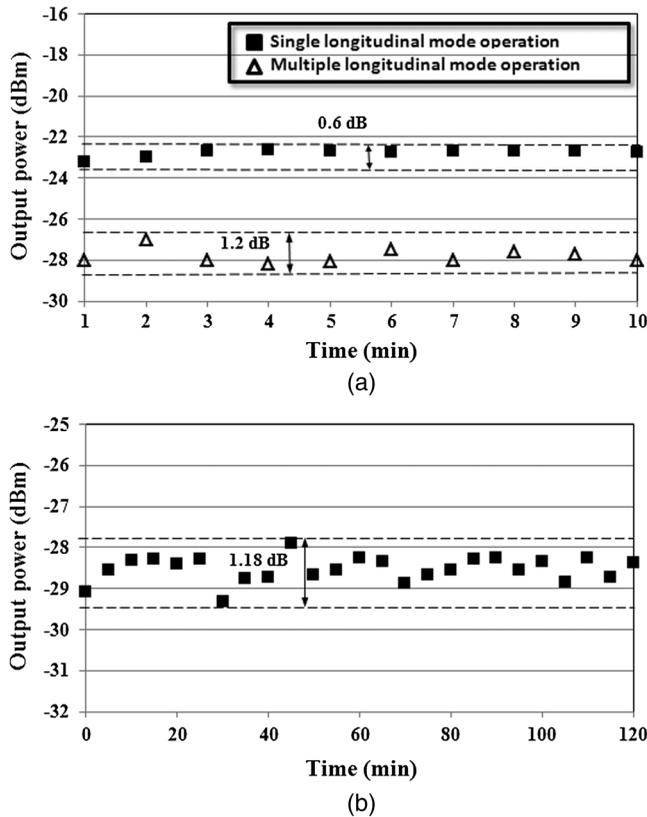
**Fig. 4** (a) Output power fluctuation for the emission line centered at 1550 nm when the laser works in single-longitudinal-mode (SLM) and multiple-longitudinal-mode (MLM) operation. (b) Fluctuation for the emission line centered at 1535 nm during 120 min when the laser operation is SLM.
