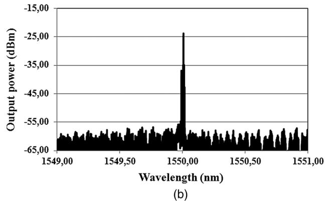
**Fig. 3** Output optical spectrum measured by the Brillouin optical spectrum analyzer for the dual-wavelength erbium fiber laser configuration when the tunable laser was tuned close to the first (a) and second (b) wavelength laser emission.
