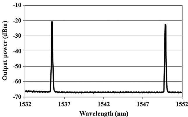
**Fig. 2** Output optical spectrum measured by the OSA for the proposed dual-wavelength erbium fiber laser for a pump power of 70 mW.
