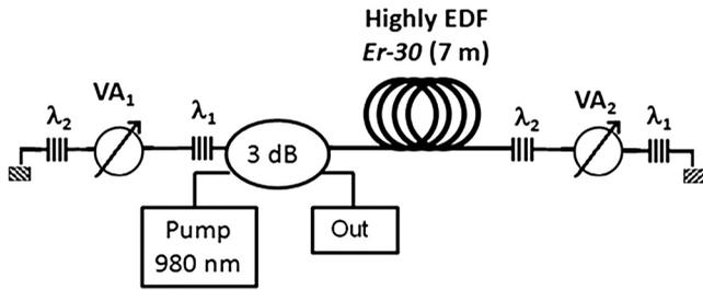
**Fig. 1** Experimental setup of a linear cavity fiber laser, where a 50% coupler is used to couple the light from a 980-nm source and to deliver the 1550-nm laser output to an optical spectrum analyzer (OSA).
