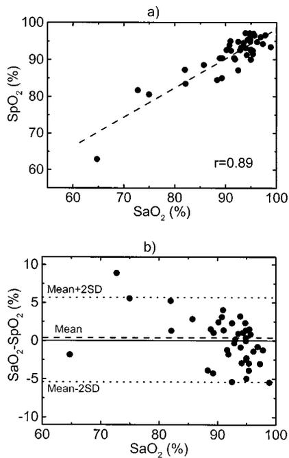
**Fig. 9** (a) Oxygen saturation  $SpO_2$  values from the NIR pulse oximetry system versus the arterial oxygen saturation obtained from the co-oximeter. (b) The corresponding Bland and Altman plot of the differences with the mean value (mean, dashed line) and two standard deviation values (mean+2 SD and mean-2 SD, dotted lines) between the two sources.
