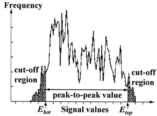
**Fig. 6** Illustration of the histogram reduction procedure. A frequency distribution of the PPG signal values is computed and a fixed sample percentage is rejected from both ends of the distribution (cutoff regions). The peak-to-peak value of the variable component  $E_{AC}$  is calculated from the difference between the maximum or higher value  $E_{top}$  and the minimum or lower value  $E_{bot}$  of the reduced-frequency distribution diagram.
