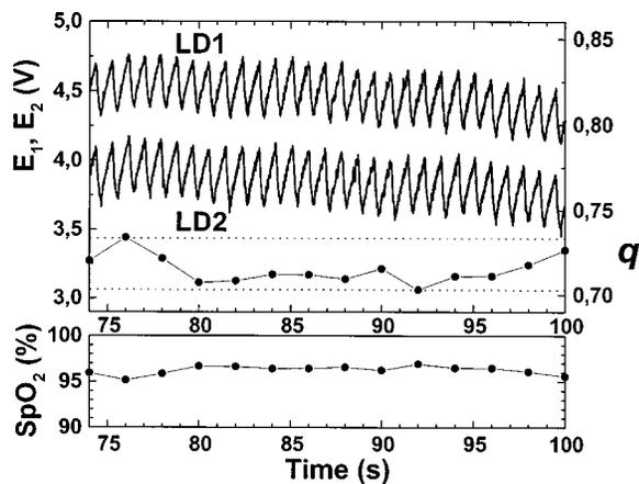
Fig. 7 Performance of the whole NIR laser diode-based transmittance pulse oximetry system at different processing stages.<sup>26</sup> In the upper part, the PPG signals corresponding to LD1 and LD2 ( $E_1$  and  $E_2$ , respectively) are represented. The middle and lower parts show the  $q$  and oxygen saturation ( $SpO_2$ ) values obtained. The dotted lines indicate the lower and higher values of  $q$  in the time interval represented.
