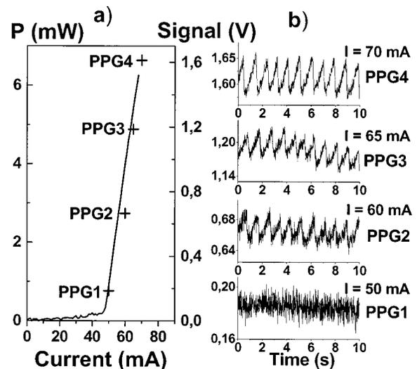
**Fig. 2** The sensor system at different emitter injection current levels in the measurement of a human pulsating vascular bed (distal part of a finger). (a) Continuous-mode power versus current characteristics (-) and the average values (+) of each PPG for the laser diode ILPN-750 in pulsed mode ( $1 \mu\text{s}$ , 1 kHz). (b) Ten seconds of PPG at different values of injection currents: PPG1 at  $I=50$  mA, PPG2 at  $I=60$  mA, PPG3 at  $I=65$  mA, and PPG4 at  $I=70$  mA.
