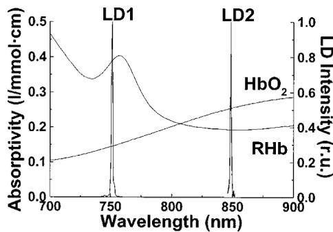
**Fig. 1** Absorption spectra of HbO<sub>2</sub> and RHB<sup>31</sup> from 700 to 900 nm and, superimposed, the emission spectra of laser diodes LD1 and LD2. The LD1 emission matches a band of local maximal differential absorption between HbO<sub>2</sub> and RHB spectra. The LD2 emission corresponds to a higher HbO<sub>2</sub> absorption than RHB.
