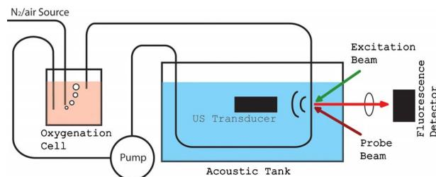
**Fig. 2** Experimental setup including a closed flow circulating dye, in plastic tubing, a peristaltic pump, and an oxygenation cell. The excitation and probe beams illuminate a section of the tubing. Photoacoustic signals are detected by a focused ultrasound transducer. Water tank is used for ultrasound coupling between the tubing and the transducer. Time-dependent fluorescent signal is detected by a photodetector and recorder using a digital oscilloscope.
