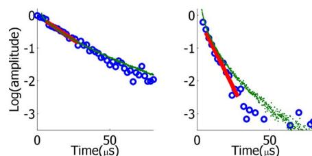
**Fig. 4** Amplitude of photoacoustic response (open circles) and fluorescence emission (dots) as a function of the time delay following an excitation pulse, for low (left) and high (right) oxygen levels. An exponential decay fit to the photoacoustic data, calculated in the range of 4 to 30  $\mu\text{s}$ , is shown (solid line).
