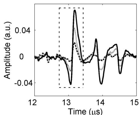
**Fig. 3** Photoacoustic signals at three different time delays (6, 34, and 100  $\mu\text{s}$ ), after a reference signal that corresponds to infinite time delay (no excitation) was subtracted. The signals were measured at a low oxygen level. The rectangular frame (dashed line) indicates the time window used for signal processing. The first and second peaks in the signals correspond to the front and back dye-tubing interfaces.
