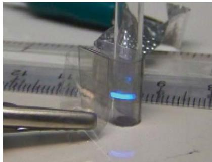
**Fig. 8** A blue PLEC bent (conformed) around a 2.5-mm-radius glass tube.
