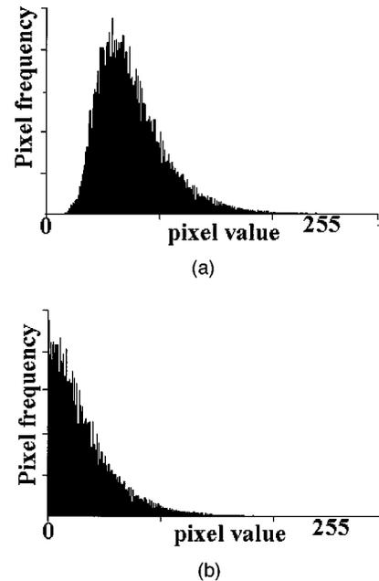
**Fig. 6** Histograms showing the probability density function of intensities in speckle on the image of a diffusing metal plate, (a) before and (b) after removing the effect of the dark current.
