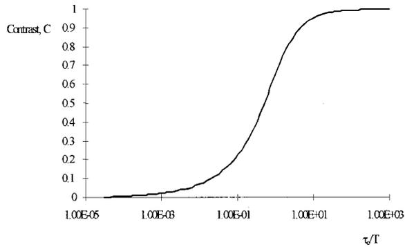
**Fig. 5** Variation of speckle contrast with the ratio correlation time to integration time for the Lorentzian model.
