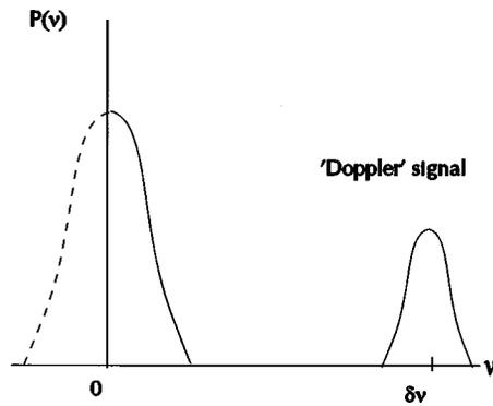
**Fig. 3** Doppler broadening (homodyne) and a separate heterodyne Doppler signal.
