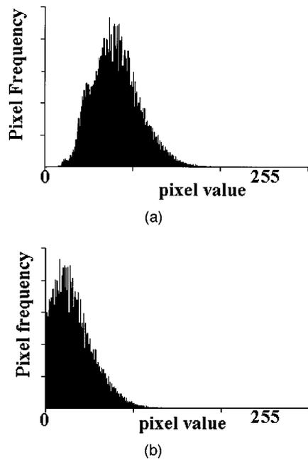
**Fig. 7** Histograms showing the probability density function of intensities in speckle on the image of a hand, (a) before and (b) after removing the effect of the dark current.
