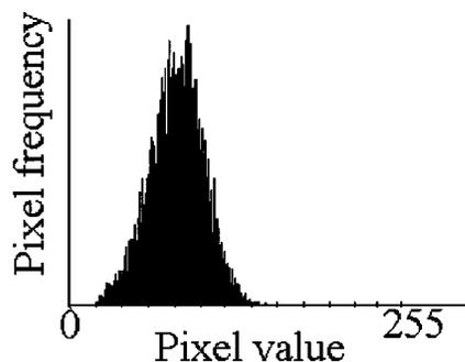
**Fig. 8** Histogram showing the probability density function of intensities in speckle on the image of a hand, after removing the effect of the dark current and ignoring the edge of the image.
