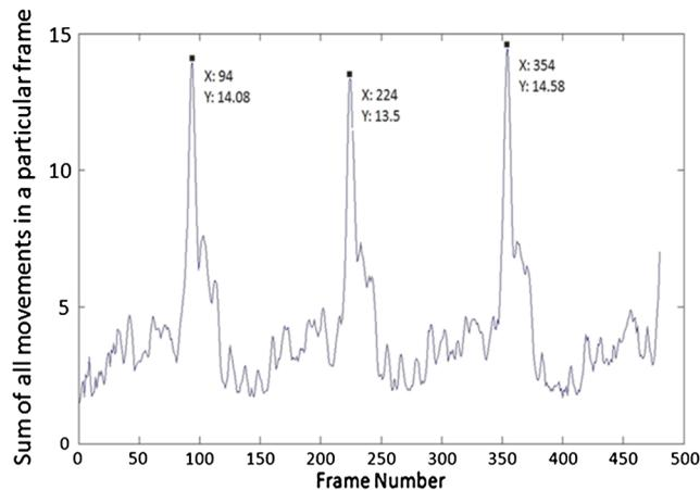
Fig. 3 Total movement (sum of movement in all squares) as a function of frame number.
