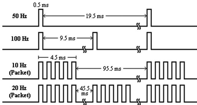
Fig. 2 Diagram showing standard (50 and 100 Hz) pulse trains compared to pulse packets (10 and 20 Hz).
