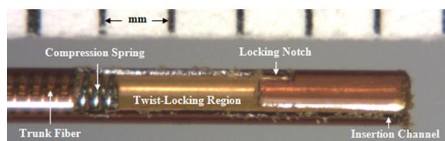
**Fig. 4** Photograph of detachable fiber tip twist-locking mechanism or “J-groove” with outer cover removed.
