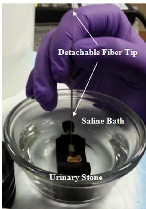
**Fig. 6** Laser lithotripsy setup consists of a human calcium oxalate monohydrate (COM) urinary stone submerged in a saline bath with the detachable fiber tip or the tapered fiber tip held manually in contact with the stone surface during laser irradiation.
