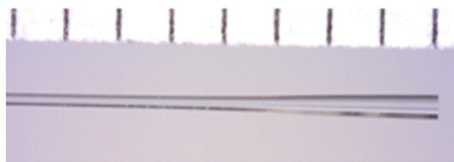
**Fig. 1** Tapered fiber distal tip used for comparative studies. Core diameter increases from  $150$  to  $300 \mu\text{m}$  over  $5 \text{ mm}$ . Scale in millimeters.
