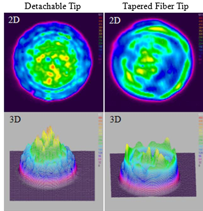
**Fig. 7** Distal fiber tip spatial beam profiles for detachable and tapered fiber tips.
