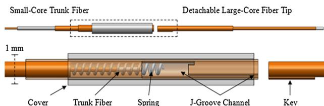
Fig. 3 Detachable fiber tip design with spring-loaded, twist-locking mechanism. The trunk fiber contains the locking mechanism while the distal tip is simply outfitted with a keyed sleeve. (Top) Overall interface and detachable tip. (Bottom) Magnified twist locking region with transparent tubing to see internal geometry.
