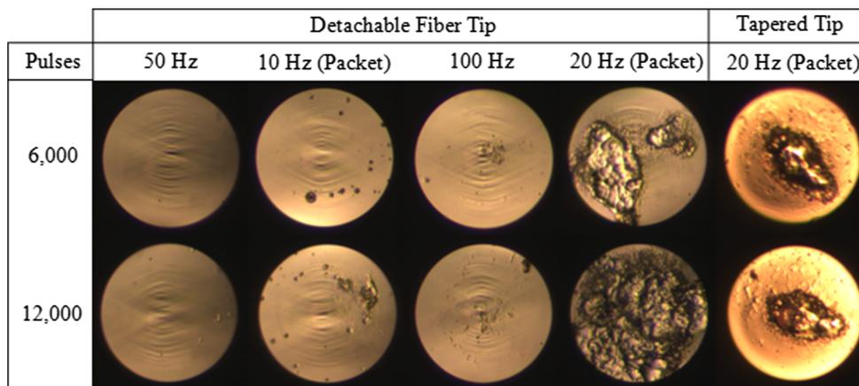
**Fig. 8** Distal fiber tip degradation as a function of pulse profile and total number of pulses. All fiber tips were held manually in contact with the stone during laser irradiation with a 30-mJ pulse energy. Considerable fiber tip degradation was observed using the 20-Hz (Packet) pulse profile for both fibers.
