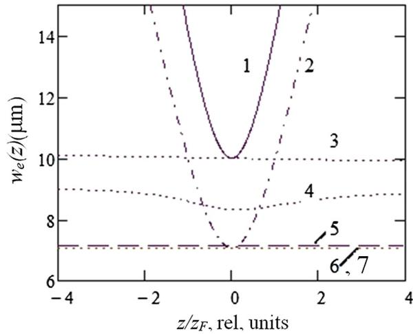
**Fig. 3** Comparison of published models (curves 1 and 2) for equivalent beam radius with the predictions of the model developed in this paper (curves 3–7; see Fig. 2 for relevant optical geometries). 1—the model of Ref. 10; 2—the model of Ref. 9; 3—free-space prediction of Eq. (11) of this paper; 4—one-lens imaging geometry for lensed fiber; 5—multiple lens optical system; 6—4f geometry; and 7—two-lens optical system.
