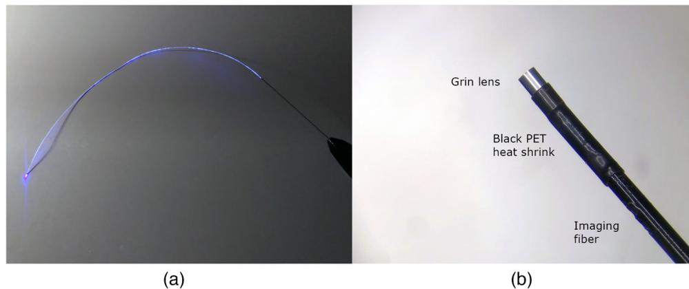
**Fig. 9** (a) Light leaks out of the thin cladding bare fiber and into fluorescent PEEK MLE. (b) Our solution was to replace the clear heat shrink covering the OD of the GRIN lens with black heat shrink.
