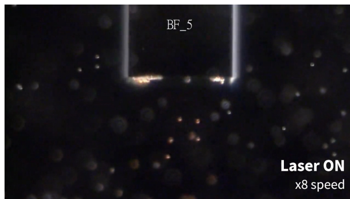
Fig. 3 5 \mu\text{m} PS particles motion under laser irradiation through different optical fibers. BF, bare fiber; GCF, gold-coated fiber; and PF, plasmonic fiber (Video 2, mp4, 9.95 MB [URL: https://doi.org/10.1117/1.JBO.28.7.075003.s2 ]).
