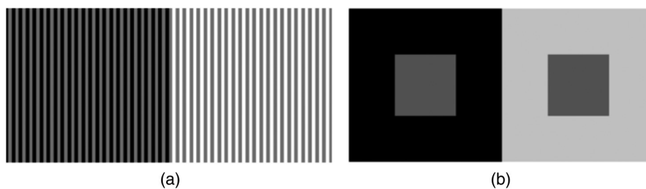
Fig 1 Lightness assimilation and contrast: (a) lightness assimilation phenomenon in which the gray bars of the same reflectance appear darker when embedded in the black bars (left) than in the white bars (right). (b) Lightness contrast phenomenon in which the gray patches of the same reflectance appear lighter inside a darker square (left) than in the lighter square (right).
