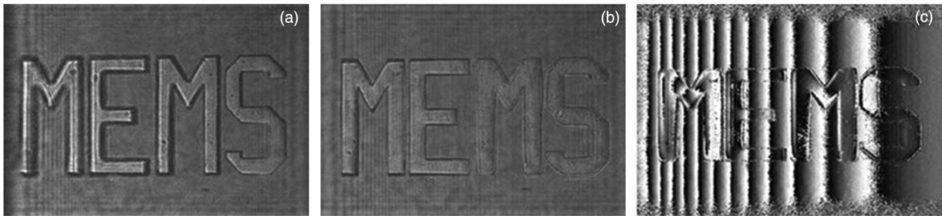
**Fig. 18** Quadratic deformation applied along the  $x$  axis to a hologram of a tilted object. (a) First frame from the video showing how EFI is got by adaptive deformation. (b) EFI image. (c) Phase difference. Images are from Ref. 81.
