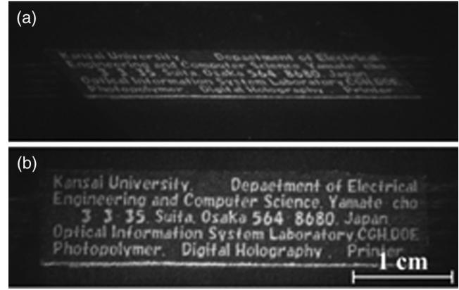
**Fig. 8** Amplitude images (a) reconstructed in the parallel plane and (b) in the tilted plane reconstructed by using rotational transformation for two-axis rotation. The planar object is rotated at  $-60$  deg around the  $x$  axis prior to rotation at 30 deg around the  $y$  axis. Images are from Ref. 63.
