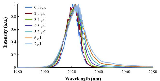
**Fig. 6** Spectrum of output pulses at various pulse energy levels after preamplifier 2.
