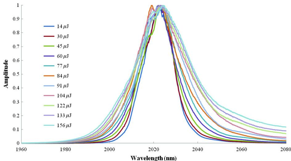
**Fig. 11** Output spectrum at various pulse energy levels.
