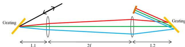
**Fig. 9** Schematic diagram of the pulse compressor.
