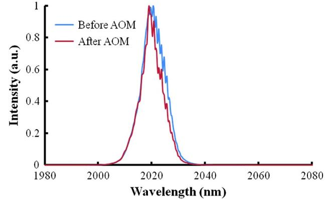
**Fig. 4** Spectra of pulses after first stage preamplifier.
