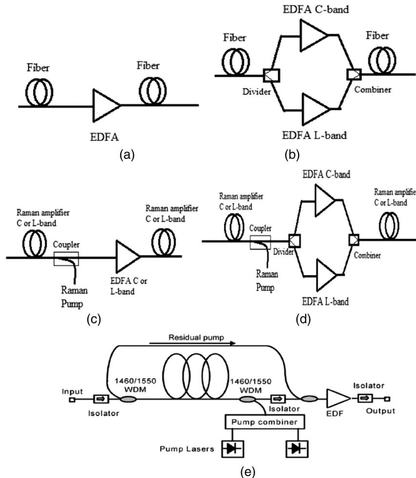
**Fig. 2** Architectures of inline optical and hybrid optical amplifiers: (a) a EDFA; (b) dual C- or L-band EDFAs in parallel configuration; (c) C + L band Raman-EDFA Hybrid optical amplifiers (HOA) in cascaded configuration; and (d) Raman-EDFA HOA, where the EDFAs are used in parallel configuration (CMB: combiner, DIV: divider); (e) cost effective Raman-EDFA HOA with residual pump.<sup>9</sup>
