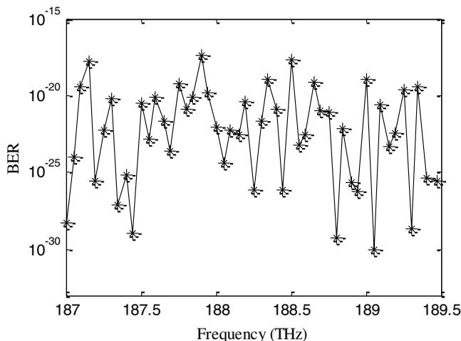
**Fig. 6** Bit error rate (BER) versus dense wavelength division multiplexed signals after transmission over EDF-Raman HOA.<sup>17</sup>
