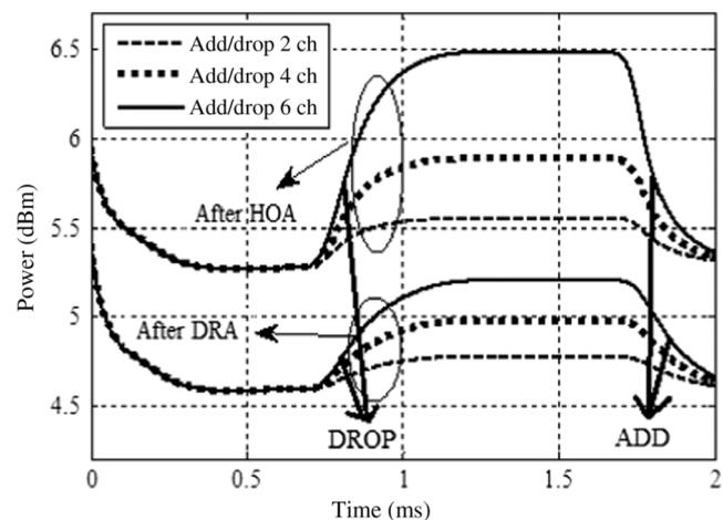
**Fig. 5** Output power of the surviving channel after distributed Raman amplifier, and HOA when 2, 4, and 6 channels are added and dropped.<sup>15</sup>
