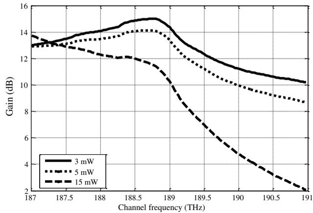
**Fig. 3** Gain spectra (with  $P_{in} = 3, 5, \text{ and } 15 \text{ mW}$ ) of Raman-EDFA HOA.<sup>42</sup>
