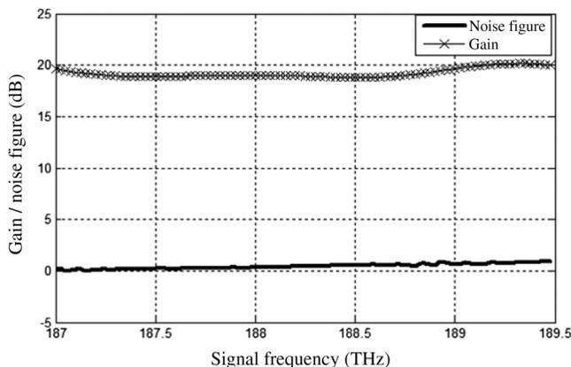
**Fig. 4** Gain and noise figure characterization of optimized EDF-Raman HOA.<sup>44</sup>
