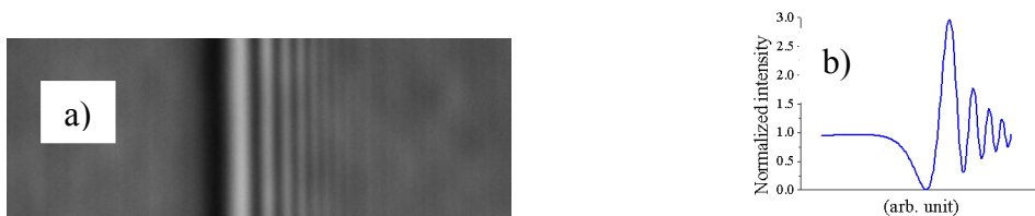
Figure 10: intensity reflected on a prism coupled to a planar waveguide. a) Measurement; b) Calculation 62 .
