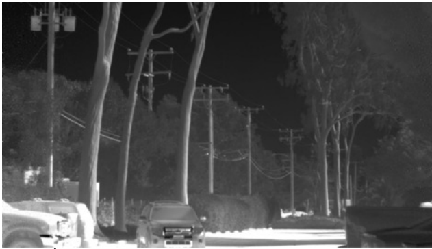
Fig. 29 Image from a HOT MWIR InAsSb array with 5 μm pixels in a 2040 × 1156 format.
