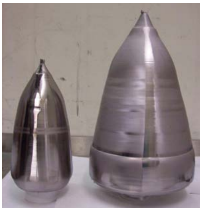
Fig. 8 Standard 2 2/3" (left) and larger format 4"-7" (right) GaSb boules.
