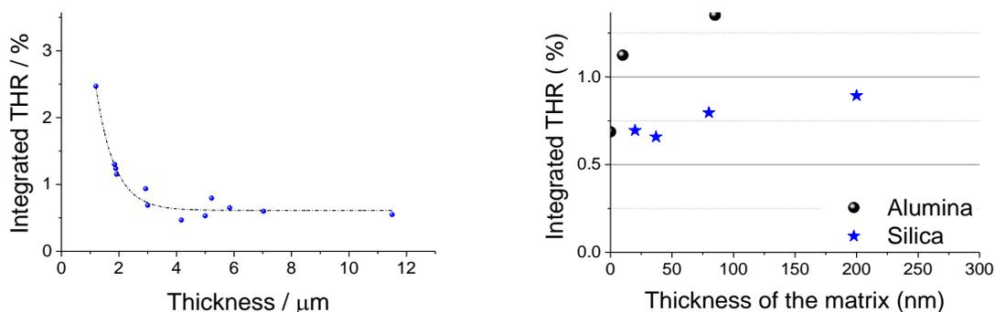
**Figure 2: Evolution of the integrated THR in the UV-Vis-NIR (300-2300 nm) as a function of the thickness of the black coating (left) and the nominal thickness of the infiltrated oxide layer (right) into a  $\sim 5\mu\text{m}$  thick CNT-based composite. (AOI:  $8^\circ$ )**
