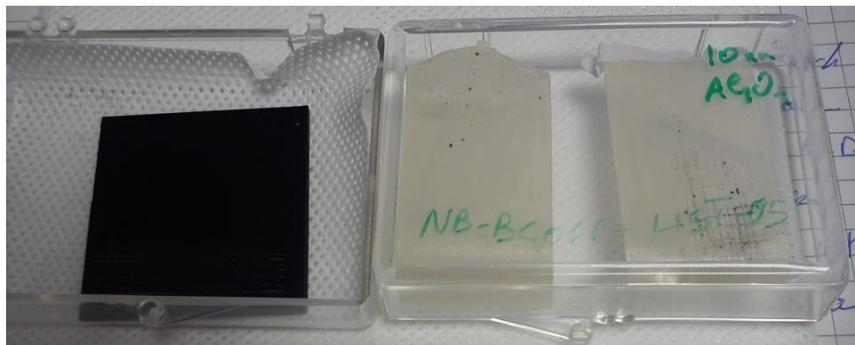
Figure 3: Adhesion/cohesion properties of coated Al sample cleaned 8 times using isopropanol and acetone soaked tissue. The black coating is reinforced in this illustration with 10nm of Al<sub>2</sub>O<sub>3</sub>
