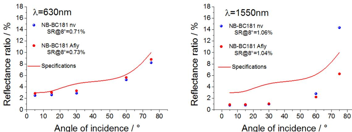
**Figure 4: TIS and specular reflection measurements of the as-grown (blue) and aged (red) black coating on Al substrate. The coating process was modified by extending the hydrolysis step in the ALD process for the growth of the  $\text{Al}_2\text{O}_3$  reinforcement layer.**
