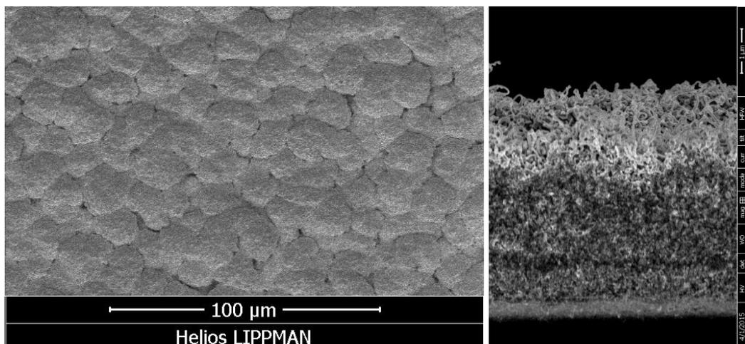
**Figure 1: SEM inspection of the surface (left) and cross-section (right) of the CNT-based nanocomposite as infiltrated by 20 nm  $\text{Al}_2\text{O}_3$ .**
