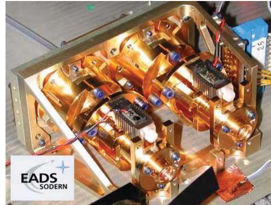
Fig. 8: Engineering Model of the ECDL.
