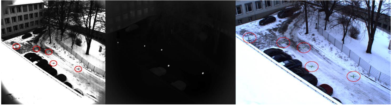
Figure 3. Calibration pattern with VSoC camera (left), IR thermal camera (center) and color camera (right). Calibration marks can be found and matched to a common coordinate system for each camera independently.
