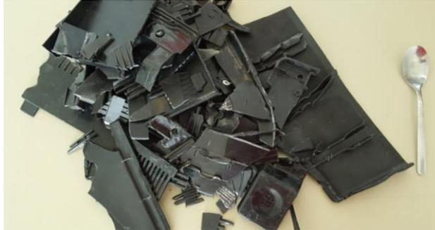
Figure 2. Roughly shredded pieces of typical black plastic waste that consists of a mixture of polymers. The tea spoon is a size indicator. (Image: inno-spec)
