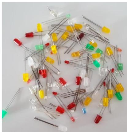
Figure 11. A collection of standard LEDs (Image: inno-spec).
