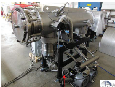
Figure 1. The vacuum pumping system (third module)
