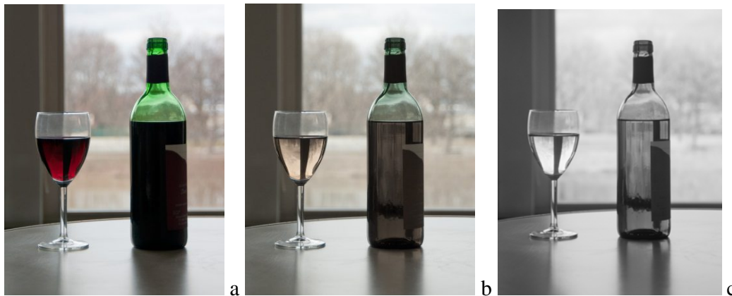
Fig. 4: Images of a bottle and glass filled with red wine recorded for VIS light only (a), whole range VIS and NIR (b) and IR only (c). Photos K. Mangold.
