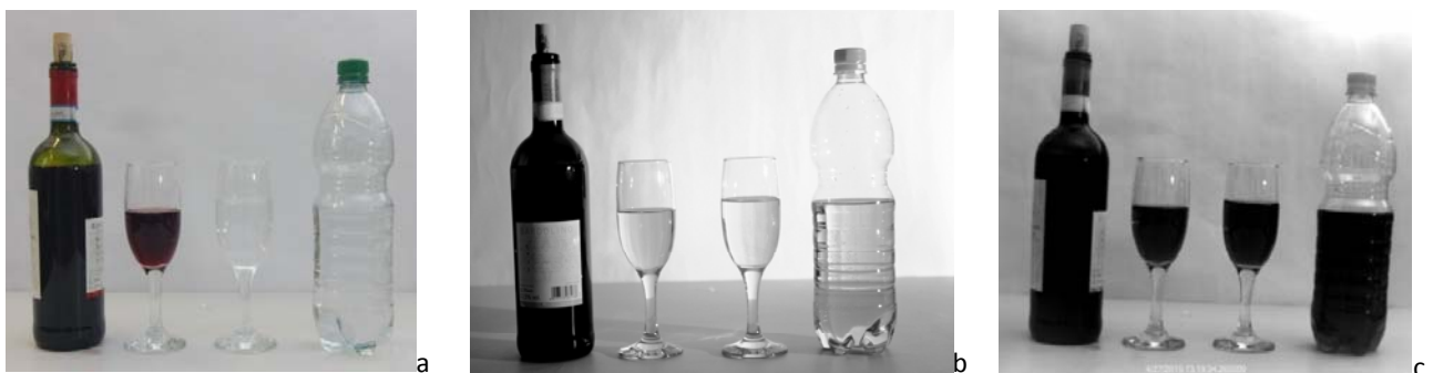
Fig. 6: Scene similar to Fig. 4 with two bottles and glasses filled with red wine (left) and water (right). a) VIS photo, (b) NIR photo recorded with Canon EOS1000 for NIR filter at cut-on wavelength 830 nm and (c) InGaAs photo..
