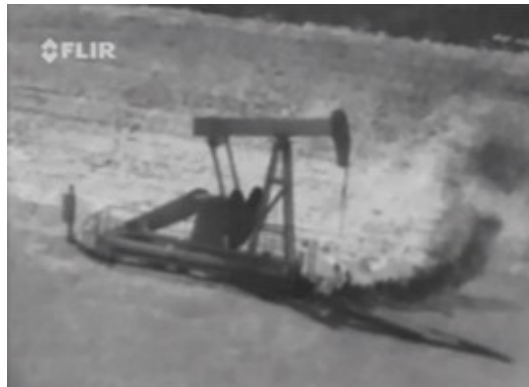
Figure 18. Airborne IR image of gas leakage from an oil well pump.
