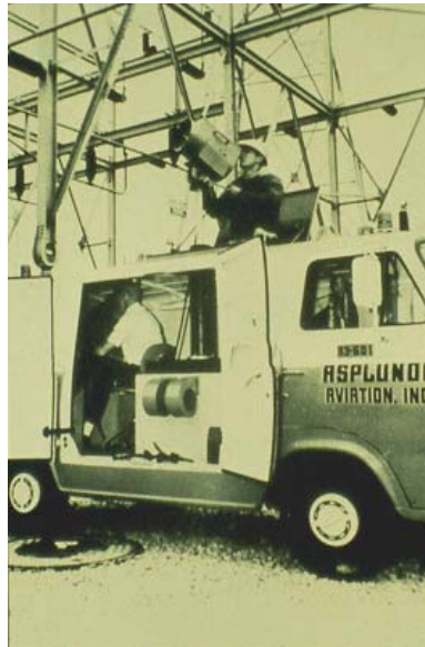
AGA Thermovision 650 mounted on inspection van
