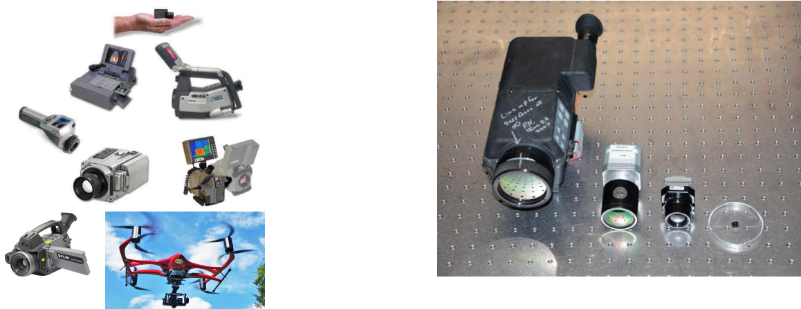
Figure 8. Left, photomontage of some 2000's era thermal imaging instruments including one on a drone. Right, uncooled microbolometer formats have decreased dramatically over time. FLIR cameras are shown from left to right: 1999 (Amber Sentinel), 2006 (FLIR Photon 320), 2013 (FLIR Tau2), and 2016 (FLIR Lepton).
