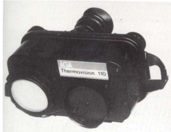
Figure 5. AGA 110 industrial thermal viewer.
