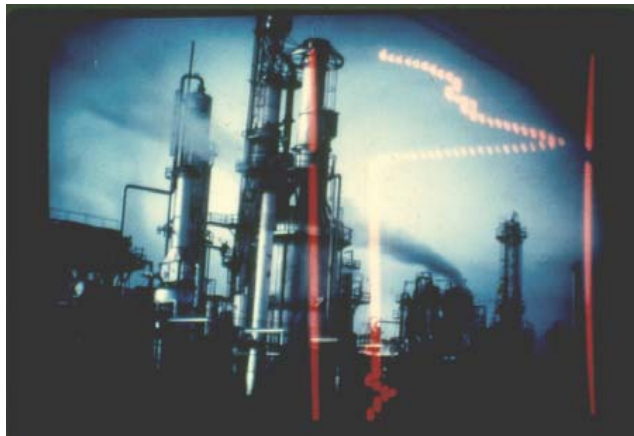
Figure 2. ThermaTrace display with vertical line scan superimposed over visible image of stack.
