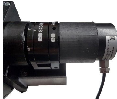
Figure 3. Measurement of the irradiance of the linear polarized incident light with a calibrated photodiode.
