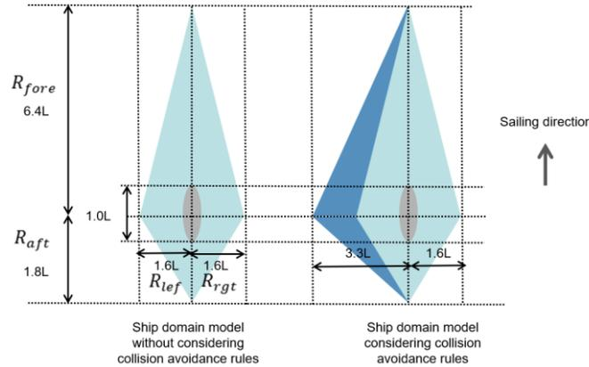
Figure 4. Two different simplified models of the ship domain.
