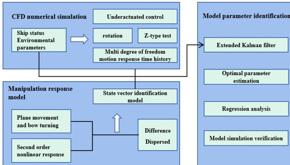
Figure 2. Overall architecture of ship manipulation response model construction.
