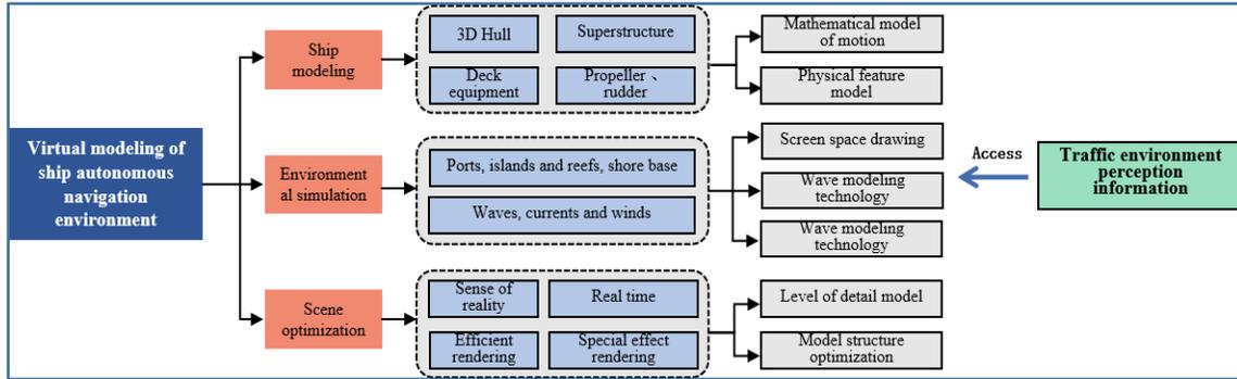
Figure 1. Overall architecture of virtual simulation modeling of ship autonomous navigation environment.
