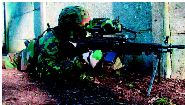
Fig. 31 Light machine gun sight with video and infrared microbolometer—from paper -97.
