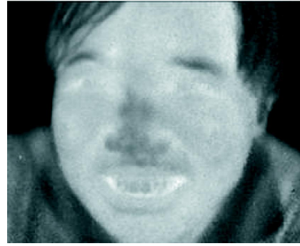
Fig. 16 Microcantilevers with an optical readout produced LWIR images in a 280x240 format as described in paper -45.
