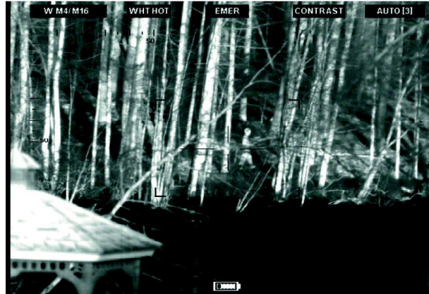
Fig. 21. Imagery from an uncooled 480 \times 640 FPA with 17 \mu m pixels from paper -59.
