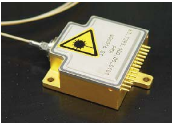
Fig. 3: Tesat Pump Laser Head, 45*45*20 mm, 150 gr, hermetically sealed
