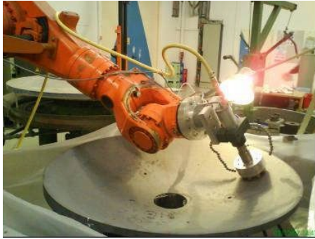
Figure 11 Antenna reflector during grinding operation
