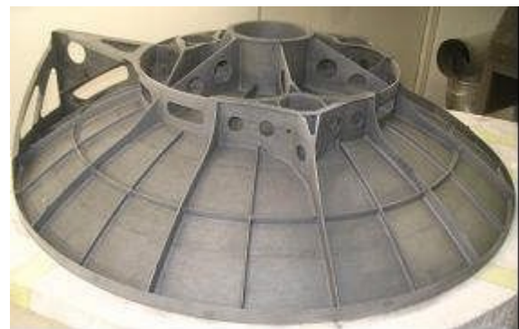
Figure 10 1 meter main reflector
