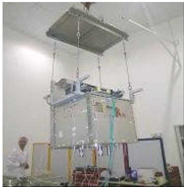
Figure 8 FM flight telescope under shock tests
