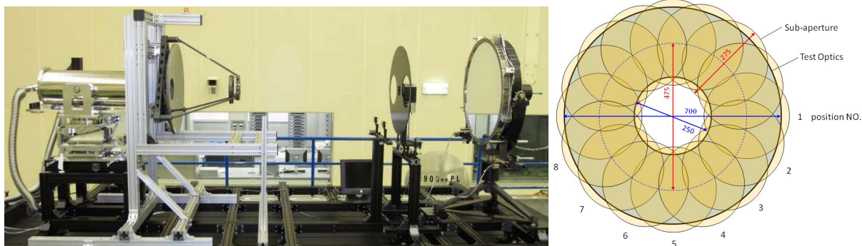
Fig. 5. (Left) Photo of the experimental configuration for the stitching interferometry before being carried into the 6-m chamber. From left to right, the interferometer in the pressure vessel mounted on the five-axis optical adjustment stage, the mirror stand, the 800-mm all-HB-Cesic telescope, the aperture mask with a rotation mechanism, and the 900-mm flat mirror with the two-axis adjustable stand. (Right) Schematics of the subapertures overlaid on the full-aperture of the \Phi 800 -mm optics.
