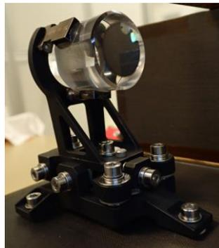
Figure 3. HRI-EUV M2 mirror with its mounting structure
