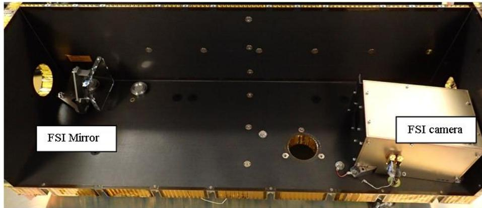
Figure 7. FSI mirror and camera on EUI OBS
