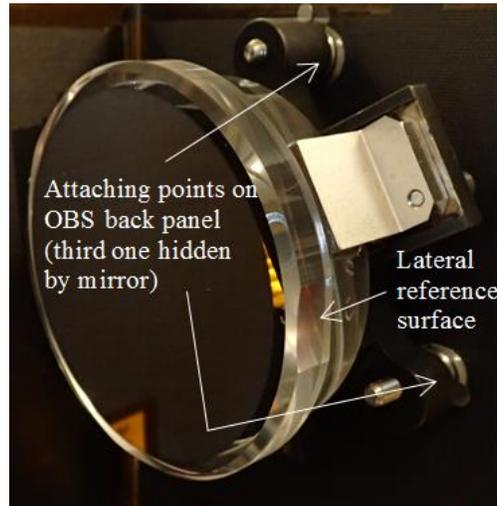
Figure 2. HRI-EUV M1 mirror with its mounting interface
