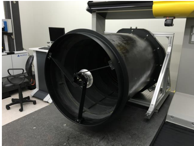
Figure 4. Alignment of M2 with respect to M1
