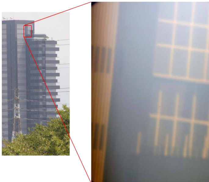
Figure 7. Imaging test of TMA telescope
