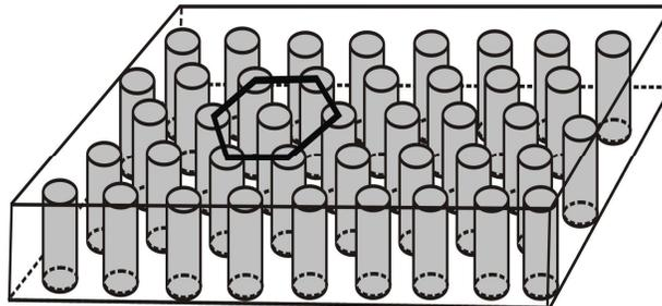
Figure 5: A nano-structure in which the columns are magnetised parallel or antiparallel to the cylinder axes. In this way the data packing density is high. Figure after ref<sup>27</sup>.
