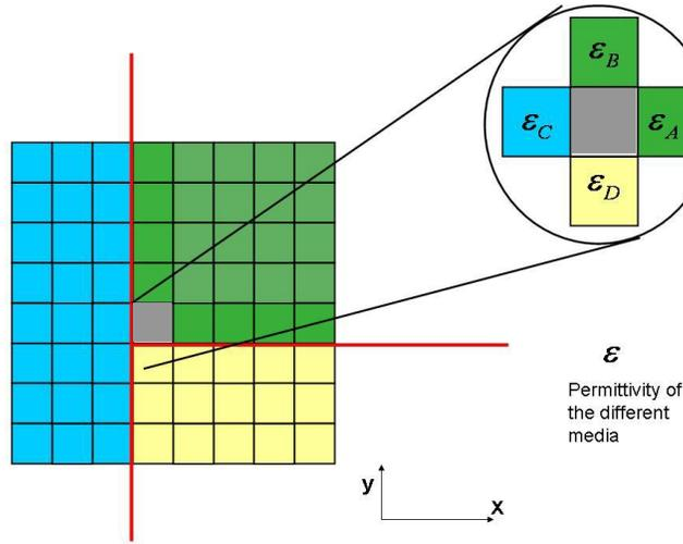
**Figure 7: Enhanced view of the neighbourhood of the corner in the end-fire configuration. The different colours signify the different permittivities.**
