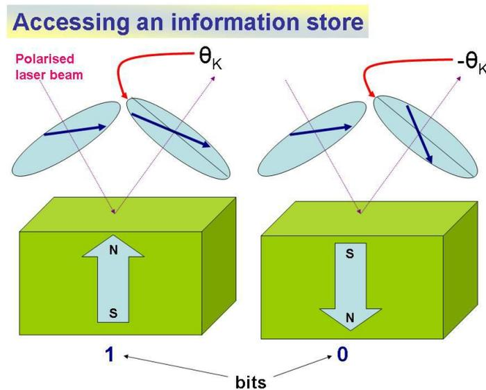
Figure 3: Elementary magneto-optic storage.  $\theta_K$  is the Kerr rotation
