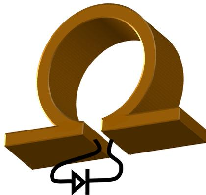
Figure 2: Omega particle equivalent circuit
