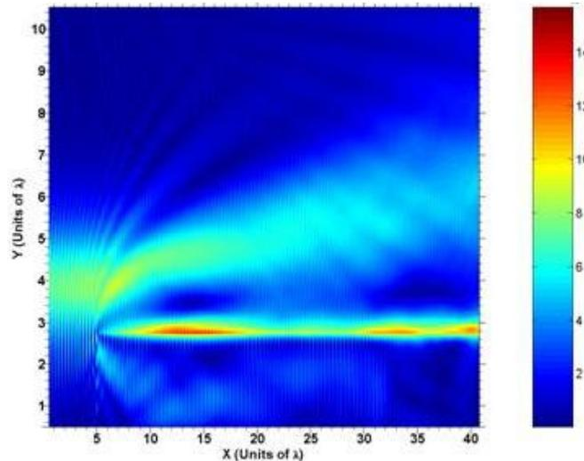
**Figure 8: Formation of a surface wave at the interface of a nonlinear material and a LHM. Number of sample points per wavelength is 100.**
