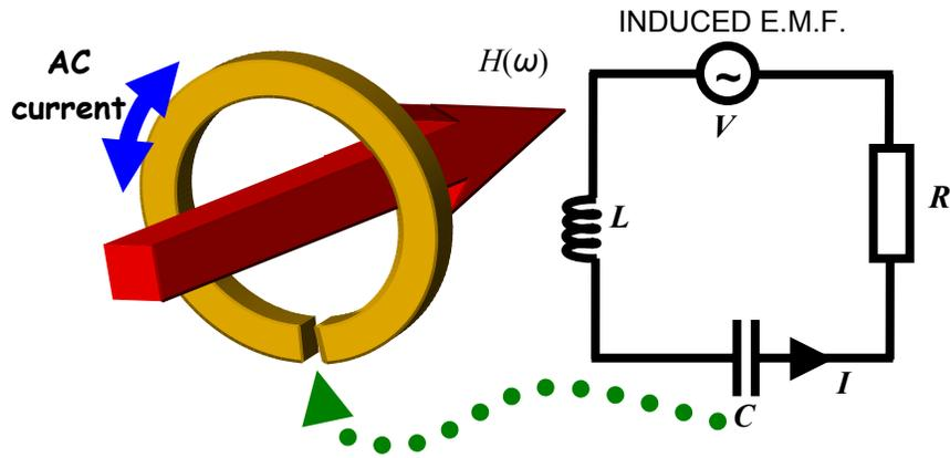
Figure 1: Split-ring equivalent circuit
