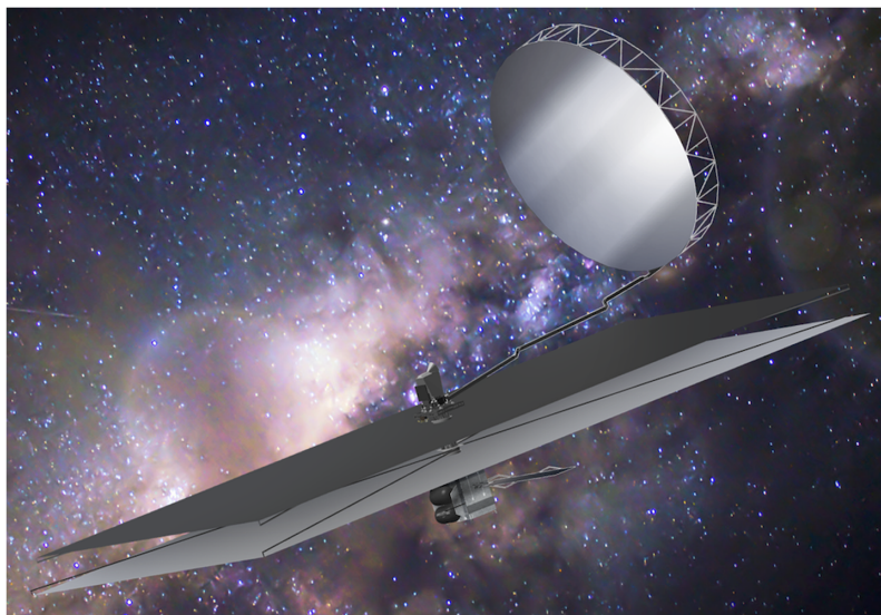
Fig. 1 SALTUS observatory uses a radiatively cooled, inflatable 14-m off-axis aperture with sensitive far-IR, high, and moderate resolving power systems to open a new window on our universe. See Sec. 3 for details on the SALTUS observatory architecture.
