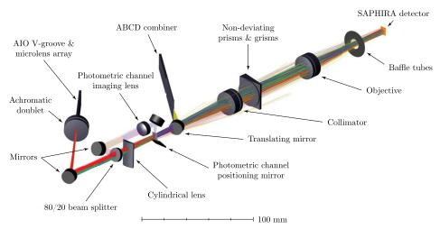
**Fig. 9** Annotated layout of the cold optic system, with beam trains for both combiners overlaid. To the left of the translating mirror are the AIO mode optics. This mirror slides out of the beam train for AIO mode observations or into the beam train for ABCD mode observations.
