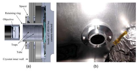
Fig. 7 (a) Position and schematic cut view of the baffle tube assembly and (b) an image of the baffle tube mounted on the inner wall of the MYSTIC cryostat. The baffle tube consists of a series of varying inner-diameter traps coated in Singularity Black paint, which absorb stray thermal background light.
