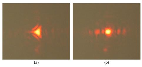
**Fig. 5** A HeNe laser signal is emitted from a fiber optic at the focal point of each OAP; the images above show the resulting collimated beam refocused by (a) an off-the-shelf OAP mirror produced by Edmund (Stock #35-491) and (b) a custom fabricated OAP by Nu-Tek. The former produces a strong coma, whereas the latter produces a smaller overall spot and does not display significant low order aberration. Both images are shown at the same physical scale.
