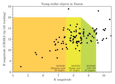
**Fig. 2** Required instrumental sensitivity to observe YSO targets in the Taurus-Auriga molecular cloud region, which drove the design specification of MYSTIC. Currently, MYSTIC as-built meets the minimum specification (orange region). Planned future upgrades (see Sec. 10) will deliver an increase of at least 1 magnitude in sensitivity (yellow region) which more than doubles the number of available objects for study.
