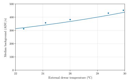
**Fig. 8** Median pixel count of the background with the detector set to a Gain of 40. By heating the external case of the dewar, we see additional thermal light coupling into the detector. The roughly fit line illustrates blackbody thermal light coupling into the camera chamber in excess of a 150 ADU/s background.
