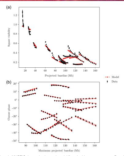
Fig. 15 Sample MYSTIC data reduction and model fit to the binary star system  $\iota$  Peg. (b) Closure phases show excellent agreement with the model binary. (a) Square visibility measurements exhibit some miscalibration, especially at the shortest baseline, which will be addressed in future versions of the data reduction pipeline.
