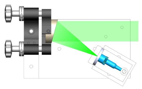
Fig. 4 Schematic view of the fiber injection mount. CHARA beams are reflected by a gold-coated off-axis parabolic mirror and focused onto a fiber tip.
