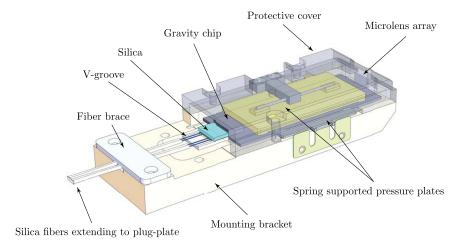
Fig. 12 Schematic of the ABCD combiner assembly prepared at IPAG. Note that the cover protecting the GRAVITY chip from incidental damage is made transparent in this diagram for illustrative purposes only.
