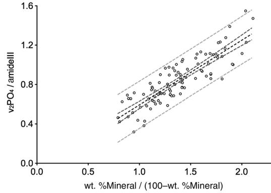
**Fig. 2** Correlation of mineral/matrix ( $v_2\text{PO}_4$ /amide III) assessed by Raman and wt. %Mineral/(100-wt. %Mineral) measured by qBEI: Each data point refers to an ROI. Additionally, the linear regression line (black dashed line), the 95% confidence bands of the slope (dark dashed line), and the 95% prediction bands (bright dashed line) are shown. As predicted by theoretical estimations, the plotted data are correlated linearly ( $R^2 = 0.75$ ).
