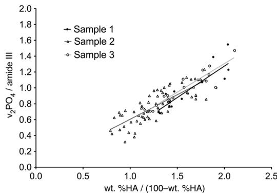
**Fig. 5** Interindividual variability: mineral/matrix versus  $\text{wt. \%Mineral}/(100-\text{wt. \%Mineral})$  are plotted for the determination of interindividual variations. Neither slopes nor intersections with the  $y$ -axis were significantly different (Sample 1: 29 years; Sample 2: 39 years; and Sample 3: 55 years).
