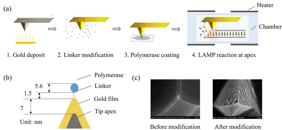
**Fig. 3** Tip preparation. (a) Undamaged tips were functionalized with MHA/EDC/NHS and polymerase. Heating plates with a temperature sensor and feedback control was covered in both sides of the chamber. (b) The distance of Au-fluorophore was estimation to be 6.6 to 7.1 nm ( $d = \text{thickness}$ ). (c) Scanning electron microscopy (SEM) image of the unmodified/modified tip.
