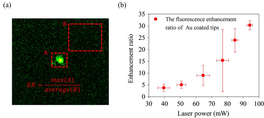
**Fig. 5** (a) Two-photon image of the tip apex under radially polarized illumination. The enhancement ratio was calculated following the formula with red color. B is a 30-pixel square and A is a random selected rectangular region including the apex image. (b) The enhancement ratio (ER) of tip apex in fluorescein isothiocyanate (FITC) solution with radial polarized illumination.
