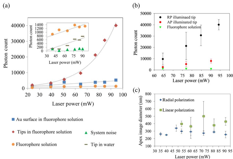
**Fig. 4** Tip strongly enhances the fluorescence. (a) Tip is with stronger emission than flat Au. Upper-left plot shows the weak background signal, which can be ignored in our experiments. (b) Effect of polarization on tip-enhanced fluorescence (TEF) signal intensity. ( $n = 5$ ). (c) The focal spot diameter is around 100 smaller with RP illumination than LP. TEF with RP illumination increased the emission intensity and made the emission spot clear to be seen.
