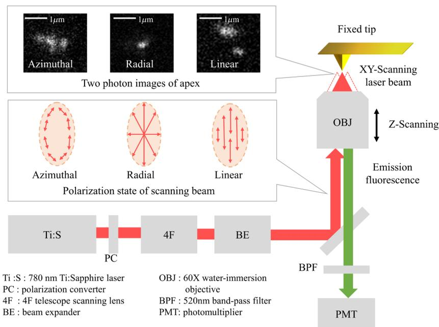
**Fig. 1** Illustration of our two-photon microscopy. The samples were scanned with three differently polarized laser beams, respectively. The upper-left image indicates the sharper focus with radially polarized illumination than the other two polarized states. The profile of the images was also affected by the shape of apices.
