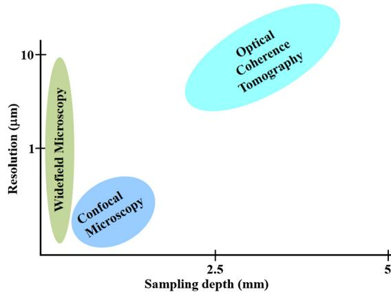
**Fig. 1** Plot of resolution versus maximum sampling depth for confocal microscopy, widefield microscopy, and optical coherence tomography imaging modalities.
