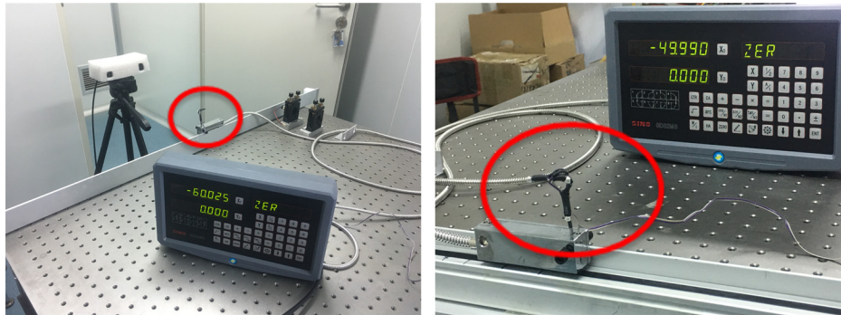
Fig. 13 Diagram of the MSI fixed on the grating ruler.
