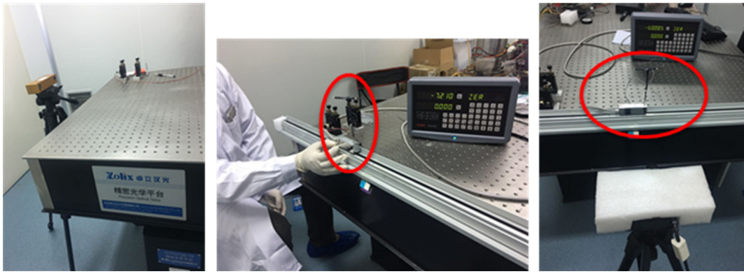
Fig. 12 Diagram of precision optical table and the TSI fixed on the grating ruler.
